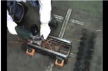
Removing weld bead and a stiffener on wall (vertical work) »
