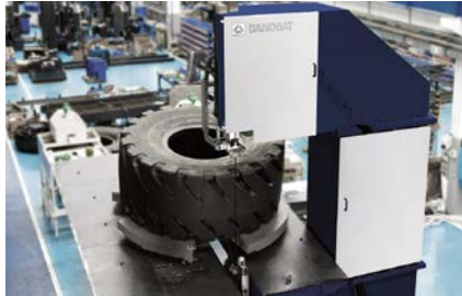
for sampling & cutting up mining tyres to facilitate disposal
